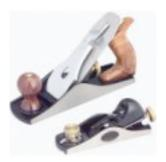
The block plane has the blade set at a very low angle so it will trim across the grain. These planes are very handy to adjust poor fitting miters when making picture frames.
