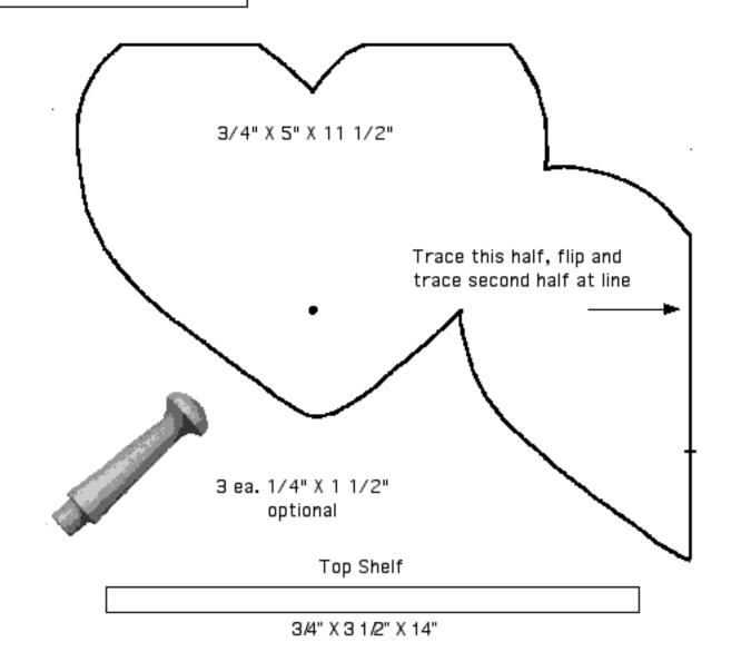
Rout keyhole slots before cutting heart shapes if you are using them, then fasten shelf to top of hearts with glue and either dowels or finishing nails, making sure these don't run into keyhole slots. Drill 1/4" holes for shaker pegs and insert them with glue.
